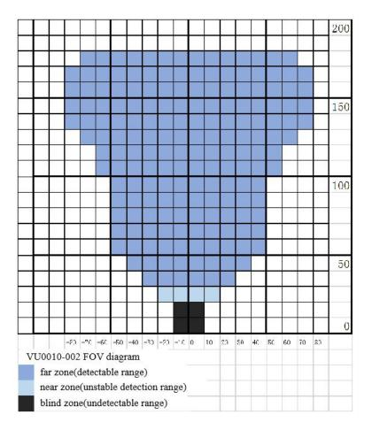
test object: 75mm standard PVC tube unit: cm
